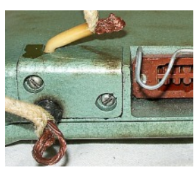
Close up view of of remote control unit socket and plug. Note the permanently attached microphone/speaker, aerial and counterpoise leads. (Serie AM)
